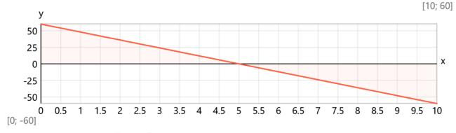
Design shear force -  $V_{\rm Ed}$  = A =  $60\,{\rm kN}$
